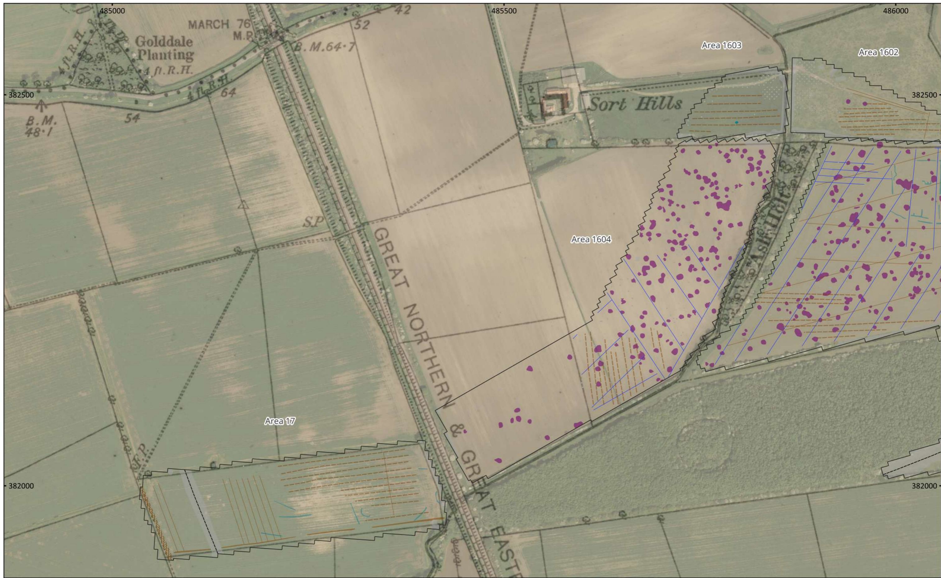
MSSK1393C - Tillbridge Solar Scheme, Cable Route, Willingham-by-Stow, Lincolnshire Figure 12 - Magnetic Interpretation Over Historical Maps and Satellite Imagery (Overview) (Areas 1603, 1604 & 17) 1:3,000 @ A3 Copyright Magnitude Surveys Ltd 2023 Contains historical mapping © CLS Data 2023: Ordnance Survey, 6" 2nd edition c. 1882-1913 Contains Satellite Imagery © Bing 2023
